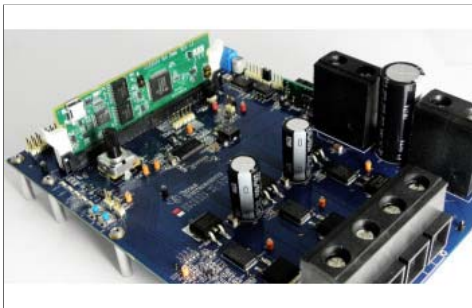
Three Phase BLDC & PMSM Motor Kit with DRV8301 and Piccolo MCU - DRV8301-HC-C2-KIT
